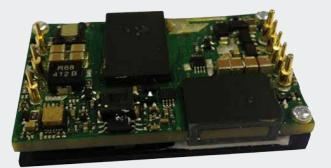
Advanced Energy's Artesyn AVQ200-36S12 series is a single output DC/DC converter with standard quarter-brick form factor and pin configuration. It delivers up to 19A output current with 12V output. Ultra-high 93% efficiency and excellent thermal performance makes it an ideal choice to supply power in telecom and datacom. It can operate over an ambient temperature range of -40°C ~ +85°C with air-cooling.
