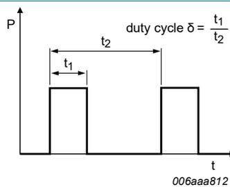
Fig. 17. Duty cycle definition
