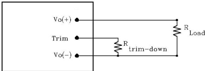
**Figure 20:** Circuit configuration for trim-down (decrease output voltage)
