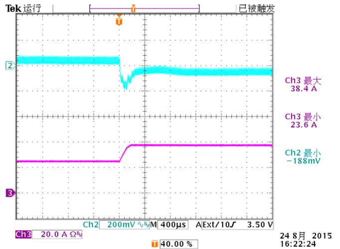
**Figure 13:** Output voltage response to step-change in load current (50%-75% of  $I_o$ , max;  $di/dt = 0.1A/\mu s$ ,  $V_{in}=54V$ ). Load cap:  $10\mu F$ , tantalum capacitor and  $1\mu F$  ceramic capacitor. Top Trace:  $V_{out}$  (200mV/div, 400us/div); Bottom Trace:  $I_o$  (20A/div, 400us/div). Scope measurement should be made using a BNC cable (length shorter than 20 inches). Position the load between 51 mm to 76 mm (2 inches to 3 inches) from the module.
