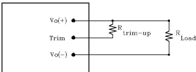
**Figure 21:** Circuit configuration for trim-up (increase output voltage)
