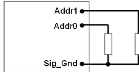
Corresponded to each octal digit, the requested resistor values are shown in below, and +/-5% resistors accuracy can be accepted. If there is any resistances exceeding the requested range, address 127 will be return. 0-12 and 40, 44, 45, and 55 in decimal address can't be used, since they are reserved according to the SMBus specifications, and which will also return address 127.
