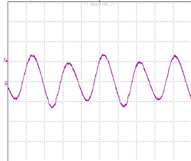
**Figure 15:** Input Terminal Ripple Current,  $i_c$ , at full rated output current and nominal input voltage with  $12\mu H$  source impedance and  $100\mu F$  electrolytic capacitor (500 mA/div, 2us/div).
