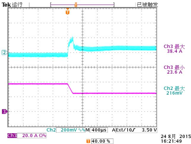
**Figure 12:** Output voltage response to step-change in load current (75%-50% of  $I_o$ , max;  $di/dt = 0.1A/\mu s$ ,  $V_{in}=54V$ ). Load cap:  $10\mu F$ , tantalum capacitor and  $1\mu F$  ceramic capacitor. Top Trace:  $V_{out}$  (200mV/div, 400us/div); Bottom Trace:  $I_o$  (20A/div, 400us/div). Scope measurement should be made using a BNC cable (length shorter than 20 inches). Position the load between 51 mm to 76 mm (2 inches to 3 inches) from the module.
