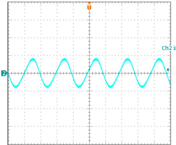
**Figure 18:** Output voltage ripple at nominal input voltage and rated load current ( $100\text{ mV/div}$ ,  $2\mu\text{s/div}$ )
