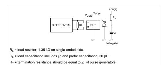
2-channel multipoint Fast-mode Plus differential I<sup>2</sup>C-bus buffer with hot-swap logic
