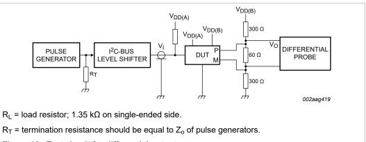
Figure 16. Test circuit for differential outputs
