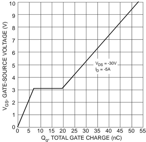
Figure 11 Gate-Charge Characteristics
