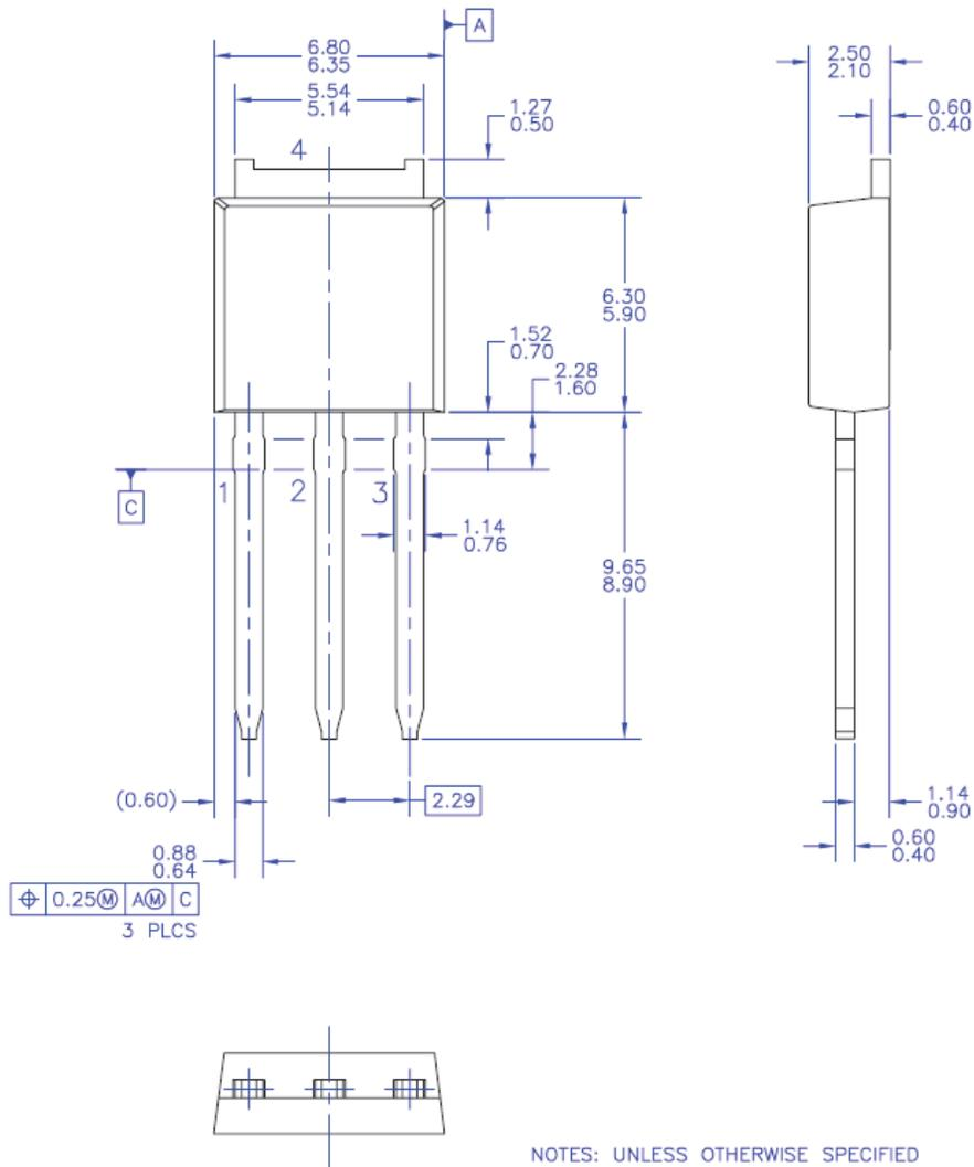
**Figure 16. TO-251 (I-PAK), Molded, 3-Lead, Option AA**
